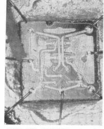
THIN FILM CIRCUITRY -Greatly enlarged photo shows a commercially-available integrated circuit approximately 1/16 in. on a side and .005-in. thick. This circuit contains six miniature conventional transistors and four resistors.
